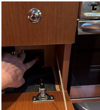
Propane solenoid switch in the galley — slide red switch down while pressing top button; green light = ON
