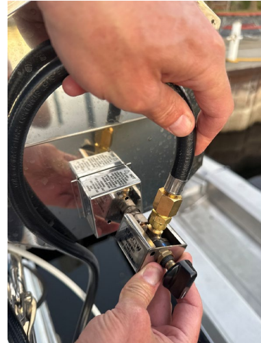
Hose connected to grill valve — rotate until snug
