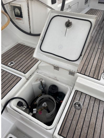
Propane locker on deck, forward of port helm — contains the tank and shutoff valve
