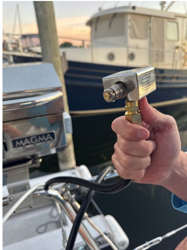
Connecting hose to the Magma grill — align the divot and push in
