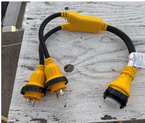
Two-30-to-50 amp converter — Only Andy to use; safe for our boat but dangerous to lend. May be needed in an old marina that can't function with the Smart Y adapter.
