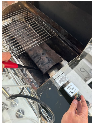
Lighting the Magma grill — use the red-handled lighter while holding the control knob
